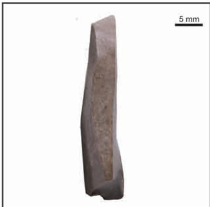
e. burin-like fracture (s-shaped fracture)
