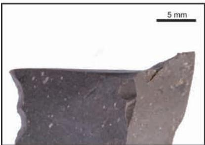
c. transverse fracture with snap termination + spin-off fractures
