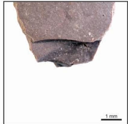
b. transverse fracture with step termination
